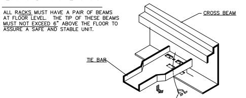
NOTE — TIE BARS MUST BE INSTALLED FOR MAXIMUM UNIT STRENGTH. ONE TIE BARS PER LEVEL FOR FOUR AND FIVE FOOT WIDTH. TWO TIE BARS PER LEVEL FOR SIX AND EIGHT FOOT WIDTH.
